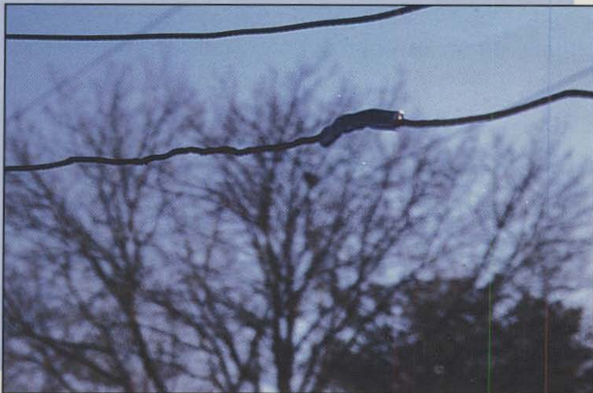
Photo E—Crimped, solderless butt connector used to extend antenna length on 10 meters, for which the wire was originally cut too short. Antenna purists probably won't like it, but it meets marine standards.
